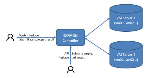
As we can see, at a high level, the system appears quite simple (although in detail, it is a highly sophisticated system). It comprises the Controller and the VM Server(s). The controller serves as the core component, it does many jobs including calling the VMs in the VM Servers for sandbox-based analysis.
