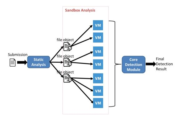
For instance, a single submitted sample may be expanded into M file objects, and each file object is dispatched to N VMs for dynamic sandboxing analysis. The final detection result is determined based on all the file objects tested across all VMs. Consequently, the total number of running VMs for a single sample is M\*N. This extensive approach ensures a more thorough and in-depth analysis compared to other sandboxing systems.
